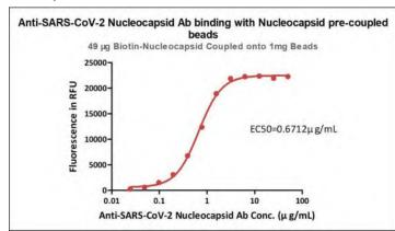
Immobilized 49 μg SARS-CoV-2 Nucleocapsid protein/1 mg beads (1 mg/mL) can bind the Anti-SARS-CoV-2 Nucleocapsid Antibody with an EC50 of 0.6712 μg/mL (QC tested).
